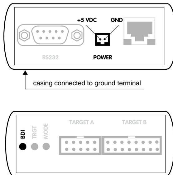
The green LED «BDI» marked light up when 5V power is connected to the BDI3000
